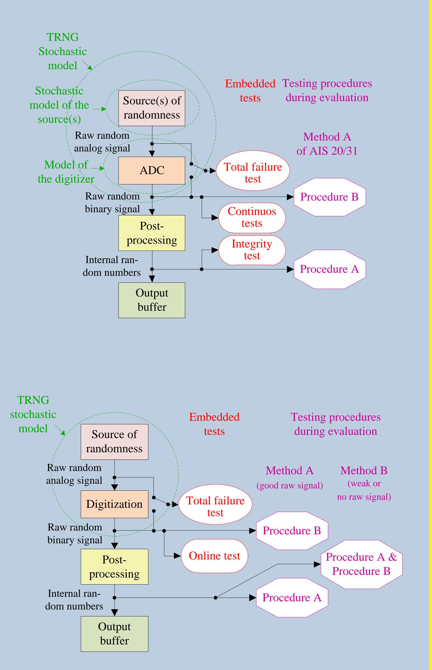
Requirement 2. ([Model] Mathematical description of the ADC) The ADC transforms elements of  $V \times S$  into a series of bits. The model of the ADC  $f_0: V \times S \rightarrow \{0,1\}^*$  describing this transformation shall be identified.
