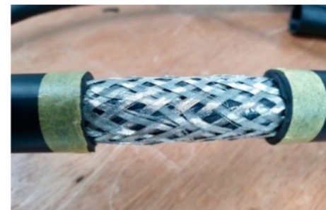
Damaged Braided Shielding
